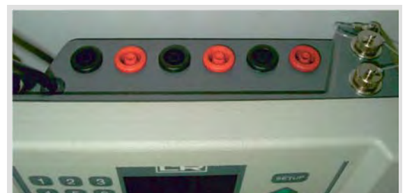
Image: Electrical ports at the LR-Cal LPC 300
